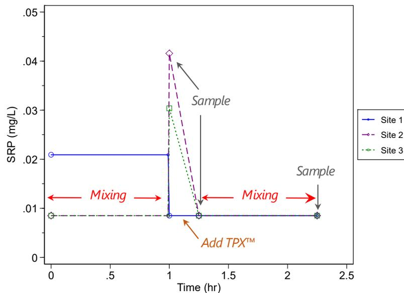
Figure 3. TPX™ mixing study showing effects of mixing (sediment resuspension) and subsequent addition of TPX™ followed by a second phase of mixing on water column SRP concentrations. Each data point represents the average of two replicates included for each site in the experiment.
