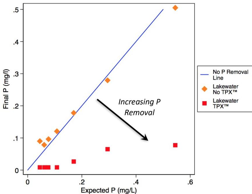
Figure 2. Adsorption isotherm showing the response between expected P concentrations in the experimental microcosm based on P spiking additions to filtered surface water from Lake Apopka (and assuming no P removal; see blue line) and the observed response in the lake water both without and with TPX™ added. TPX™ dose was 100 mg/L.
